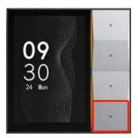
You can configure the button function by going to > Button Settings, selecting the desired button and tapping to choose the relay or scene to be controlled.
