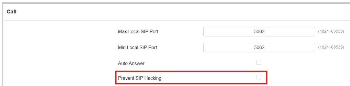
The screenshot shows the 'Call' settings page. It includes fields for 'Max Local SIP Port' (5062, 1024~65535) and 'Min Local SIP Port' (5062, 1024~65535). There are checkboxes for 'Auto Answer' and 'Prevent SIP Hacking'. The 'Prevent SIP Hacking' checkbox is highlighted with a red border.
