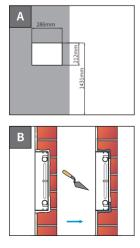
Cut out a square hole on the wall with the dimension 212\*286\*42mm (height\*width\*depth).
