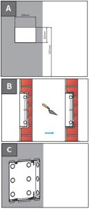
Cut out a square hole on the wall with the dimension 209\*188\*40mm (height\*width\*depth).
