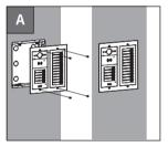
Use the **Torx wrench** to tighten the device with four **M4x15 Torx head screws.** Installation is completed.
