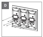
Fasten wiring cover with M2.5x6 crosshead screws.
