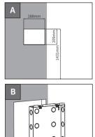
Cut out a square hole on the wall with the dimension 209\*188\*40mm (height\*width\*depth).
