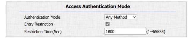
• **Restriction Time(Sec)**: Specify the time within which the same user cannot open the door twice. For example, if it is set to 1800 seconds, the user cannot open the door again until 30 minutes later.
