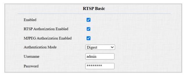
MJPEG Authorization Enabled: Once enabled, accessing the door phone's real-time image or video by entering the URL into the browser requires verification of the Authentication Mode, User Name, and Password.
