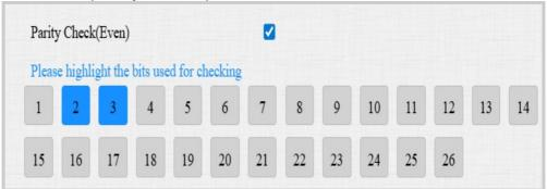
• Parity Check(Odd): When enabled, the sum of selected bits must be odd to pass verification. For example, when the second and third bits are selected and their sum is odd, the parity check passes.
