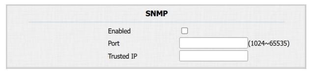
• **Trusted IP**: The allowed SNMP server address. It can be an IP address or any valid URL domain name.
