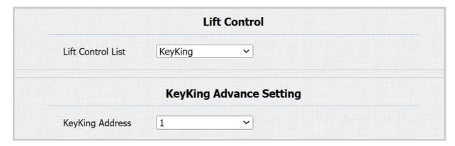
• **KeyKing Advance Setting**: Select the number from 0 to 126. The binary number converted from the address number corresponds to the dip switch on the lift board. For example, if you select 5, set the dip switch to 101000.
