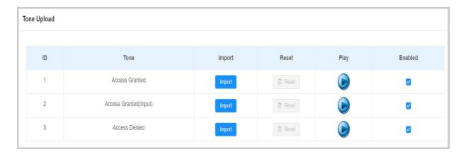
• Access Granted(Input): The door is opened by pressing an exit button connected to the device's input.
