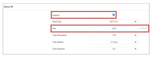
• **Port**: Set the port for direct IP calls. The default is 5060, with a range from 1-65535. If you enter a value within this range other than 5060, ensure consistency with the corresponding device for data transmission.
