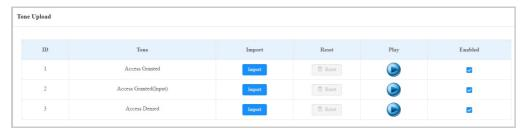
• Access Granted(Input): The tone is played when the door is opened by pressing an exit button connected to the device's input.
