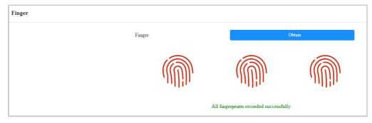
Place the user's finger that is used to open the door in the fingerprint reader area. The same fingerprint needs to be recorded three times.
