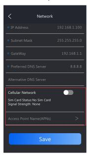
• Access Point Name(APNs): You can press this option to add new APNs. Fill in the information from your network provider.
