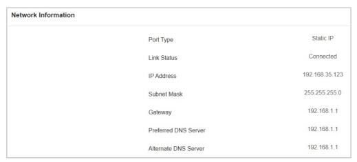
Set the network connection on the web Network > Basic interface.
