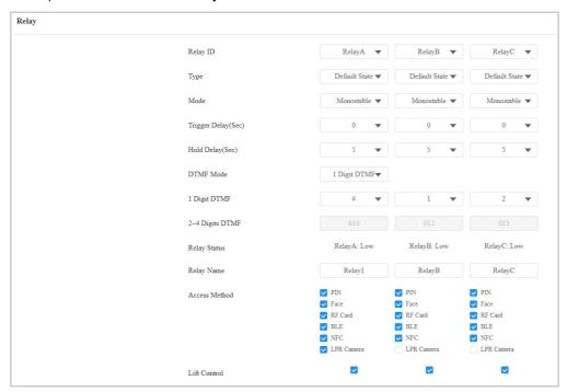
Relay ID: The specific relay for door access.
