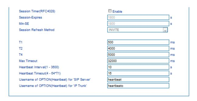
Figure 3.10-3 SIP Parameter Configuration Interface
