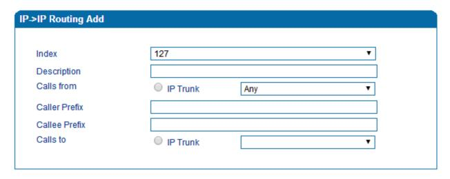
Figure 3.11-7 Configuration Interface for IP->IP Routing
