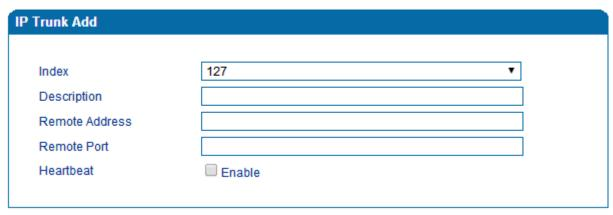
Figure 3.11-3 IP Trunk Configuration Interface
