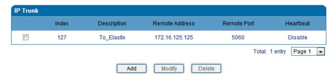
As shown above, the IP trunk is created, and the remote end IP address is 172.16.125.125, the SIP port is 5060.
