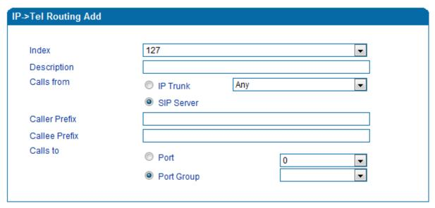
Figure 3.11-5 Configuration Interface for IP-Tel Routing
