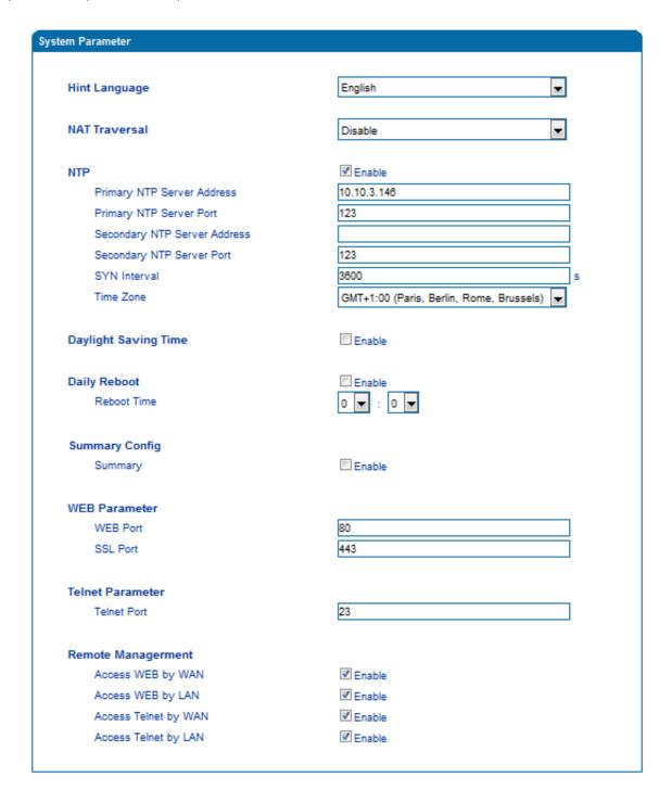
Figure 3.10-7 Configuration Interface for System Parameters
