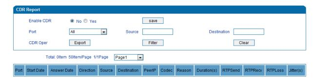
On the **Status & Statistic CDR** interface, details of all calls through the ports of the DAG2500-72S are displayed. The CDR function can be enabled on this interface.
