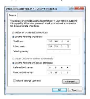
Check the connectivity between the PC and the gateway. Click **Start**  $\rightarrow$  **Run** of PC and enter cmd to execute 'ping 192.168.11.1' to check whether the IP address of the DAG2500-72S gateway runs normally.
