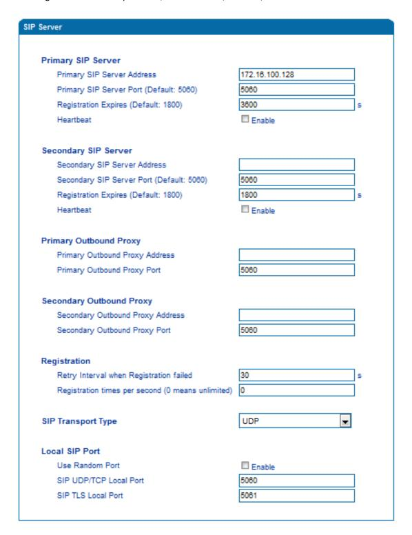
Figure 3.8-1 Configuration Interface for SIP Server
