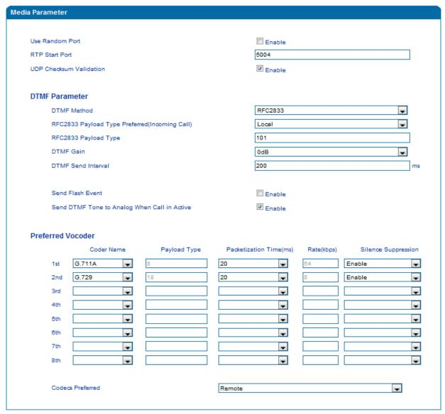
Figure 3.10-2 Configuration Interface for Media Parameters
