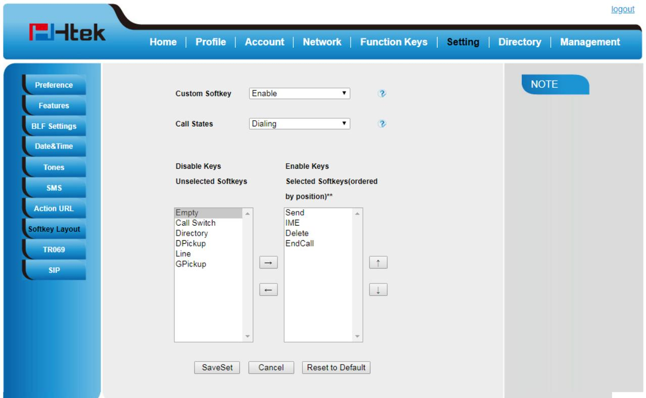
The screenshot shows the Htek web interface for configuring the Softkey Layout. The top navigation bar includes Home, Profile, Account, Network, Function Keys, Setting, Directory, and Management. The left sidebar lists various settings: Preference, Features, BLF Settings, Date&Time, Tones, SMS, Action URL, Softkey Layout (selected), TR069, and SIP. The main content area shows the following configuration options:
