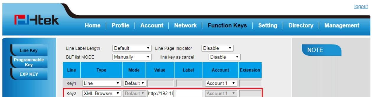
The screenshot shows the Htek web interface with a navigation menu at the top: Home | Profile | Account | Network | Function Keys | Setting | Directory | Management. On the left, there are buttons for Line Key, Programmable Key, and EXP KEY. The main content area displays configuration options for Line Keys. A table lists the configured keys, with Key2 highlighted in red. The table has columns for Line, Type, Mode, Value, Label, Account, and Extension.
