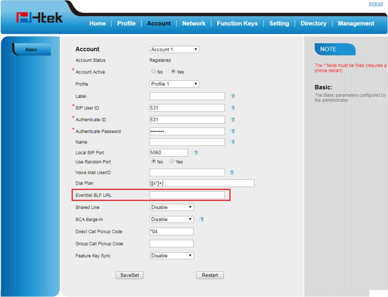
The screenshot shows the Htek web interface for configuring an account. The 'Basic' tab is selected in the sidebar. The 'Account' section contains various fields for configuration. The 'Eventlist BLF URL' field is highlighted with a red box. The 'SaveSet' button is visible at the bottom of the form. A 'NOTE' section on the right states: 'The \* fields must be filled (requires a phone restart)'. Below the note, it says 'Basic: The Basic parameters configured by the administrator.'
