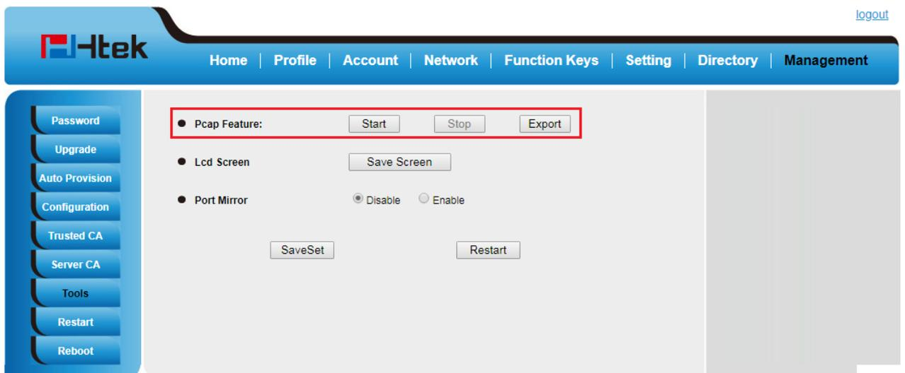
The screenshot shows the Htek web interface with the 'Pcap Feature' section highlighted in a red box. The interface includes the same navigation and sidebar as the previous screenshot. The main content area shows the 'Pcap Feature' section with 'Start', 'Stop', and 'Export' buttons. Below it are 'Lcd Screen' and 'Port Mirror' sections with their respective controls. 'SaveSet' and 'Restart' buttons are also visible at the bottom.
