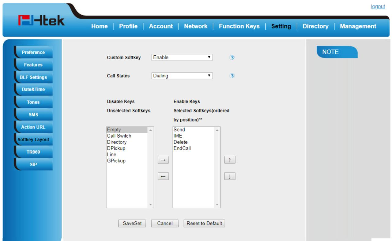
The screenshot shows the Htek web interface for configuring Softkey Layout. The top navigation bar includes Home, Profile, Account, Network, Function Keys, Setting, Directory, and Management. The left sidebar lists various settings: Preference, Features, BLF Settings, Date&Time, Tones, SMS, Action URL, Softkey Layout (selected), TR069, and SIP. The main content area shows the following configuration options:
