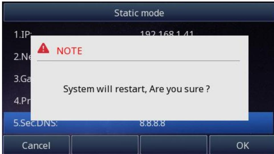
4. Press the OK soft key to accept the change or the Cancel soft key to cancel. If you are using an xDSL modem, you can connect your phone to the Internet via PPPoE mode. You can set a WAN port to be a PPPoE port. The PPPoE port will perform a PPP negotiation to obtain the IP address. Contact your system administrator for the PPPoE user name and password.
