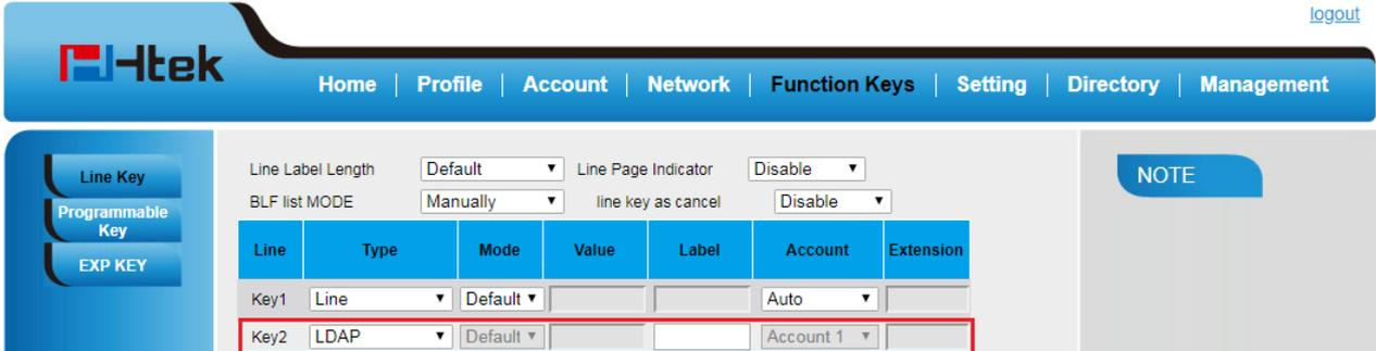
The screenshot shows the Htek web interface for configuring a Line Key. The navigation menu includes Home, Profile, Account, Network, Function Keys, Setting, Directory, and Management. The 'Function Keys' section is active, showing options for Line Key, Programmable Key, and EXP KEY. The configuration form includes fields for Line Label Length (Default), Line Page Indicator (Disable), BLF list MODE (Manually), and line key as cancel (Disable). A table lists the configured keys:
