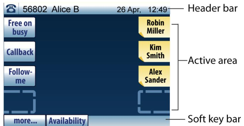
Figure 2: Example of a display in idle mode
