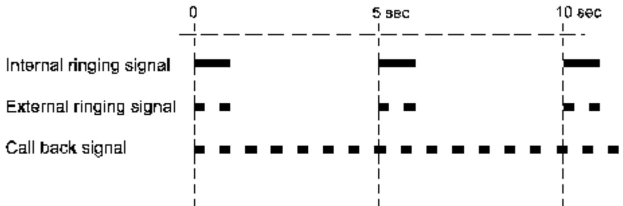
Figure 9: Ring Signals Characteristics
