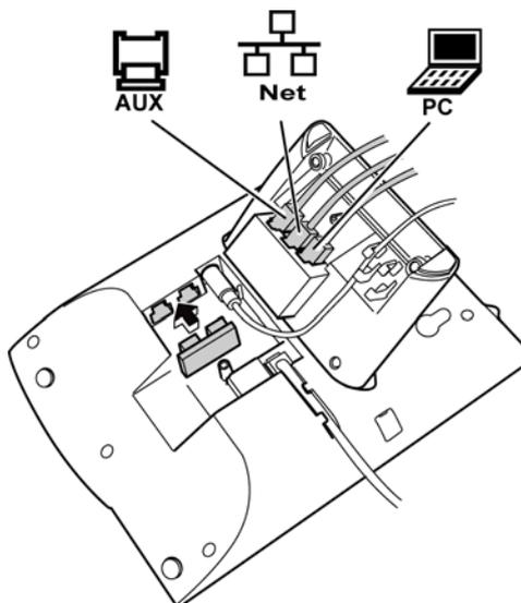
**Note:** Unless the LAN cable is connected to the port marked **Net** on the option unit, the phone will not work.
