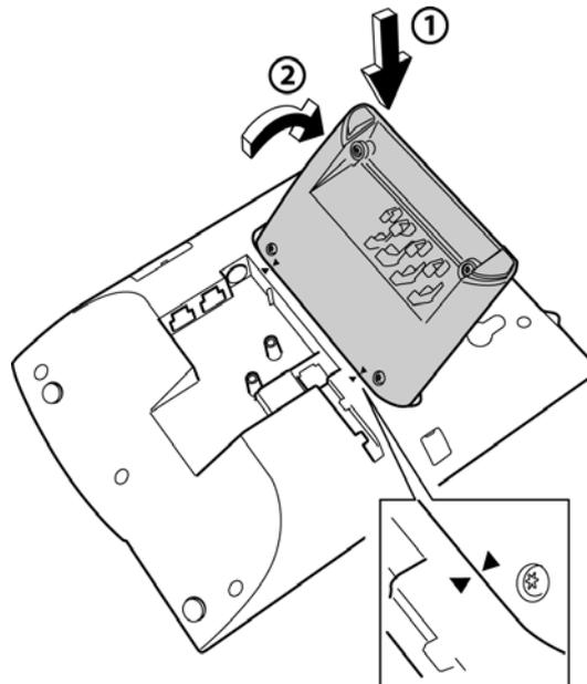
**Note:** If you wish to remove the foot console, pull the console firmly towards you to release it before removing it from the phone.
