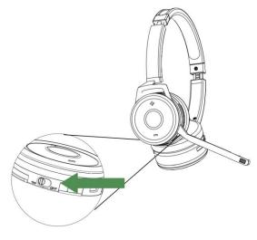
Hold (2 secs) the On/off/connect switch in the connecting position
