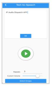
TTS paging on the IP Audio Dispatch App is different with TTS paging on the IP Audio Dispatch Console. On IP Audio Dispatch Console, TTS is used to create triggered paging, including immediate, timetable and dial number triggered paging. On IP Audio Dispatch App TTS is used for immediate paging, users can page the text contents right after the converting from text to speech.
